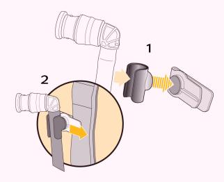
First Use Attach the tube holder to the tube(1). Attach the universal clip to the shoulder strap on your backpack or your shirt(2) and pull it up to the valve. Magnet both together.
